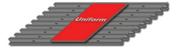
U=Uniform load – lb/ft or kg/mtr of width ΔU=Uniform load deflection (in or mm)
