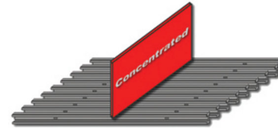
C=Concentrated line load – lb/ft or kg/mtr of width ΔC=Concentrated line load deflection (in or mm)
